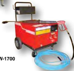
*Model OEPW-1700:* Optional Electric Pressure Washer is heavy-duty commercial grade. Comes with magnetic motor starter and industrial rocker on/off switch for pump motor with auto start/stop function. Wand assembly is stainless steel with variable pressure, 4 quick disconnects, stainless steel nozzles, and down-stream detergent injector. 230V/240V, 3 phase AC power, 10HP motor.
